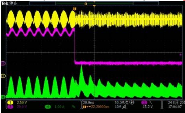
LED Short Fault Happen (CH1-VDD, CH3-VLED, CH4- Inductor Current)
