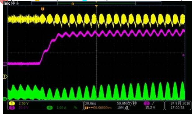
LED Short Fault Recovery (CH1-VDD, CH3-VLED, CH4- Inductor Current)
