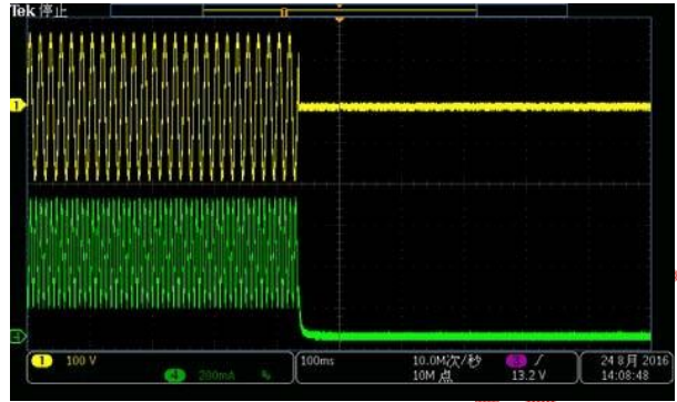
System Shut Down (CH1-VINAC, CH4-LED Current)
