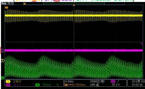
LED Short Fault Steady State (CH1-VDD, CH3-VLED, CH4- Inductor Current)
