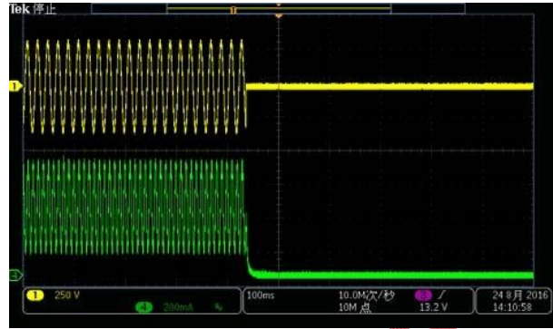
System Shut Down (CH1-VINAC, CH4-LED Current)
