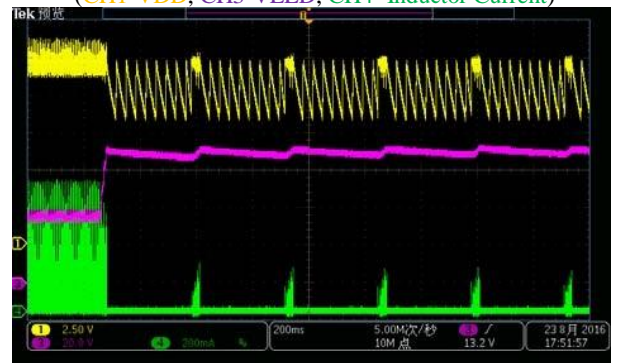
LED Open Fault Happen
